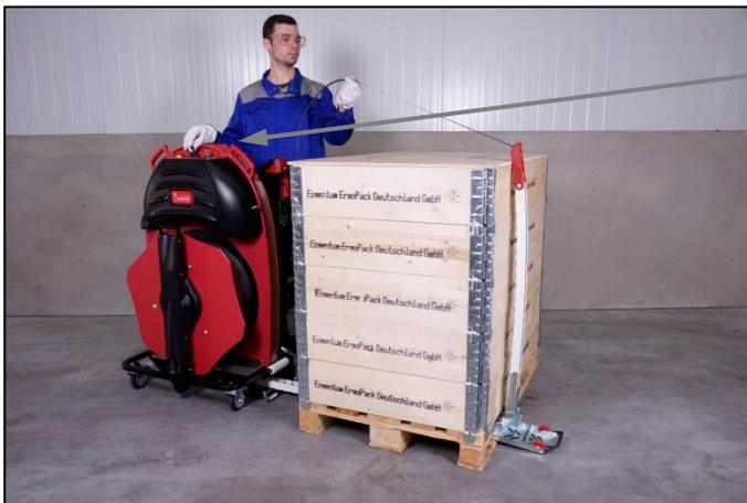
... move the ChainLance completely back by pushing the joystick in „move in“ direction.
