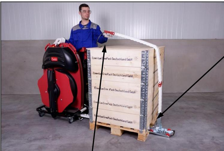
If the setting of the pallet width and the positioning of the strapping system are correct, the distance between the chain and the pallet is about 10 cm.
