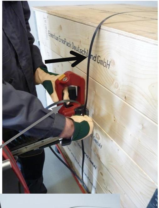
Pull the rocker lever to open the clamp of the sealing head.
