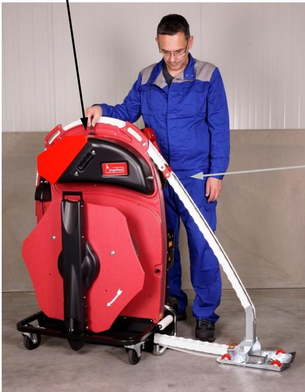
...and continue to move out the ChainLance until the red chain link is at about the same level as the left handle of the system.
